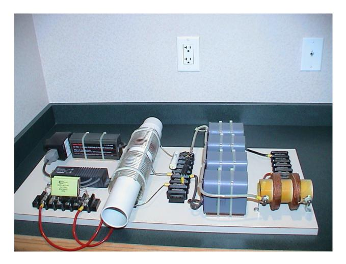
The battery supplies a small current through a protecting diode, to a standard off-the-shelf "true sine-wave" inverter.
