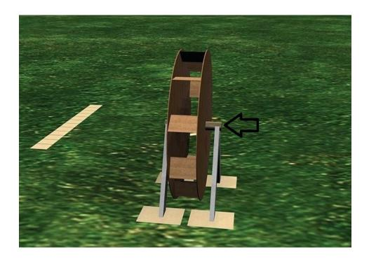
The spin of the generator will be independent from the water wheel because of the clutch. Once the speed of the water wheel will reach 300 RPMs, the spins of the wheel will simply add to the spins of the Hoon generator and provide an even bigger voltage that will result in more KW from your generator. The One-Way Ratcheting Dog Clutch will provide the extra spin for the generator as the driveshaft of the generator will maintain the minimum constant of 300 RPM.
