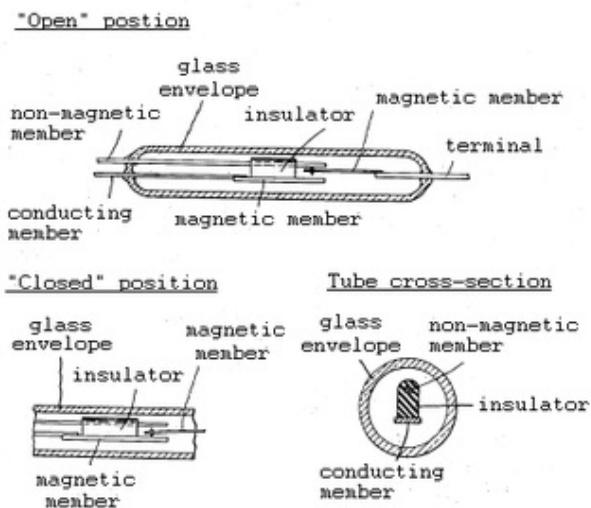
a magnet close to it. Once the magnet is pulled away from the switch, the reed switch will go back to its original position.
