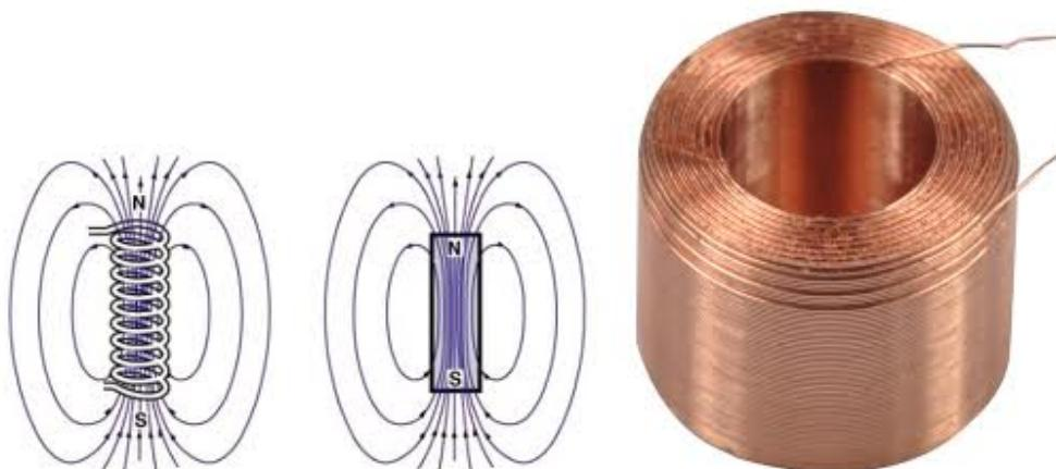
The direction of the magnetic field of a coil can be determined using the right-hand rule. If the fingers of the right hand are curled around the coil in the direction of current flow (conventional current, flow of positive charge) through the windings, the thumb points in the
