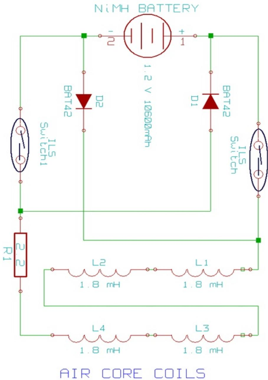
The ceramic resistor 2.2 ohms is used to reduce the current flow in the coils
