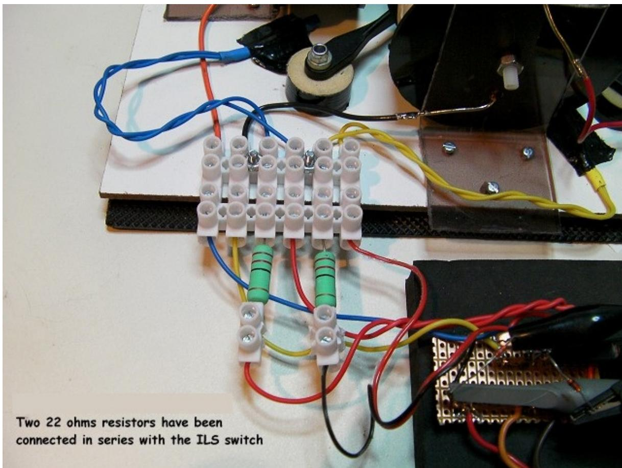
Two 22 ohms resistors have been
