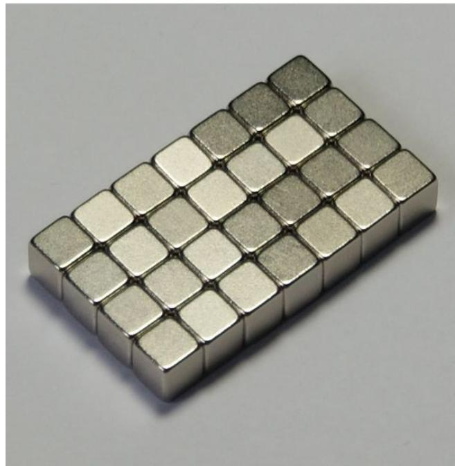
Neodymium magnets have replaced alnico and ferrite magnets in many of the myriad applications of the modern products that require strong permanent magnets, such as motors in cordless tools, hard disk drives, and magnetic fasteners.
