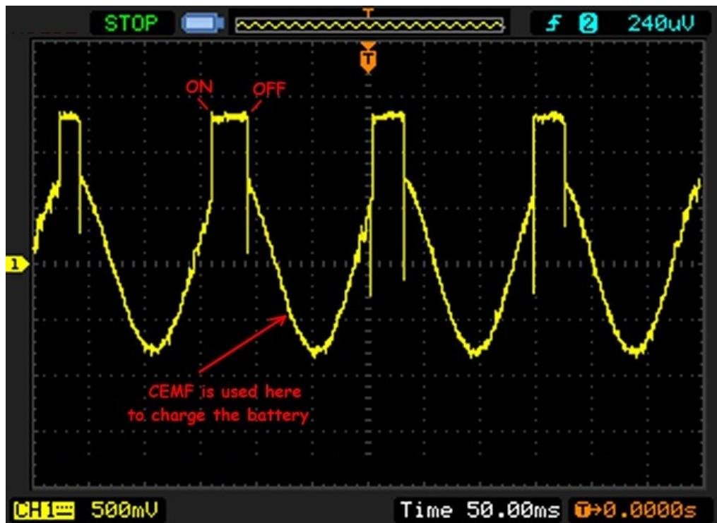
Above, the voltage across the coils: Timing is very important here, the 1st ILS switch is used to set the start of the pulse, the 2nd ILS switch is used to set the end of the pulse. Shorter the pulse is, better the efficiency... The CEMF induced in the air coils by the strong Neodymium magnets is used here to charge the battery, so the motor is able to self-charge its own battery through the fast switching and low voltage drop.
