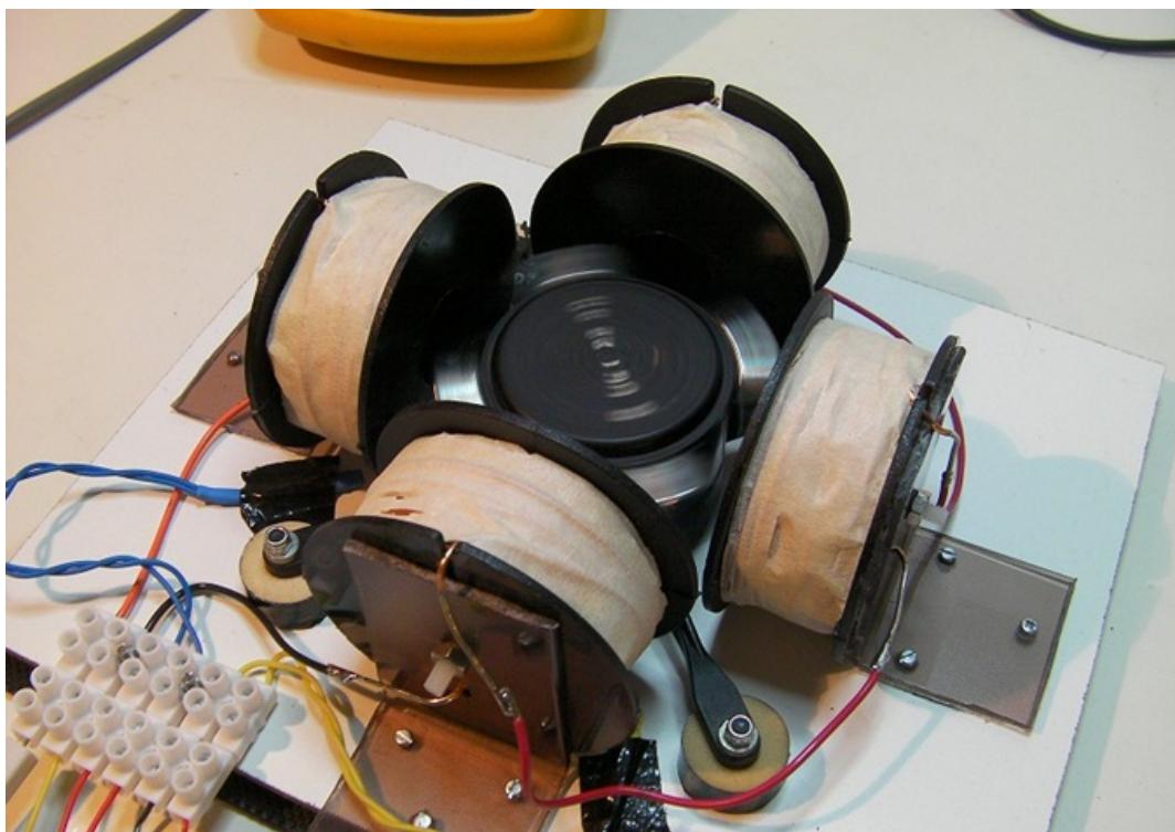
The "Brandon motor" uses four AIR CORE coils and four NdFeB magnets mounted on rotor.
