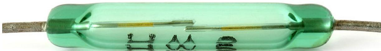
The reed switch contains a pair (or more) of magnetizable, flexible metal reeds. The end portions are separated by a small gap. The reeds are hermetically sealed in opposite ends by a tubular glass envelope. One important quality of the switch is its sensitivity.
