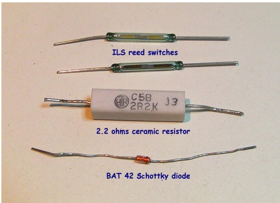
**BAT 42 schottky diode:** is used for general purpose applications. These diodes feature very low turn-on voltage and fast switching. These devices are protected by a PN junction guard ring against excessive voltage, such as electrostatic discharges.
