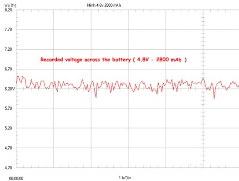
To reduce the duration of the battery voltage measurement, I have used a 4.8V NiMh battery (2800 mAh) (photo below),
